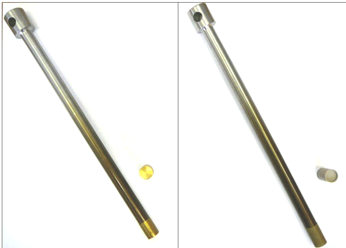
FIGURE 3. Comparison between conventional copper piston tip (left) and PEEK piston tip (right) for the RH7-2 capillary rheometer.
