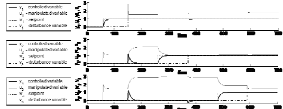
Fig. 4. Simulation course of control loop with utilization of method of desired model
