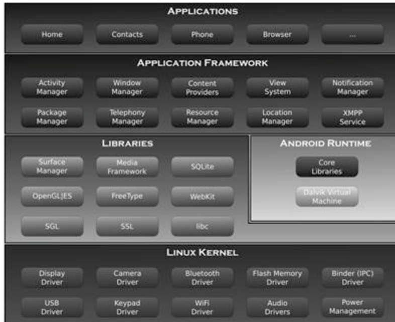
Figure 2: An Android operating system architecture diagram; (Wang, 2012), modified
