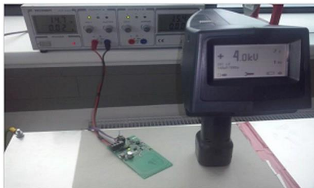
Fig. 3. The functional sample of the RFID reader and the ESD generator ONYX 16 [5]
