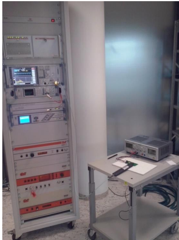
Fig. 4. Measurement of the RFID reader’s antenna radiation pattern
