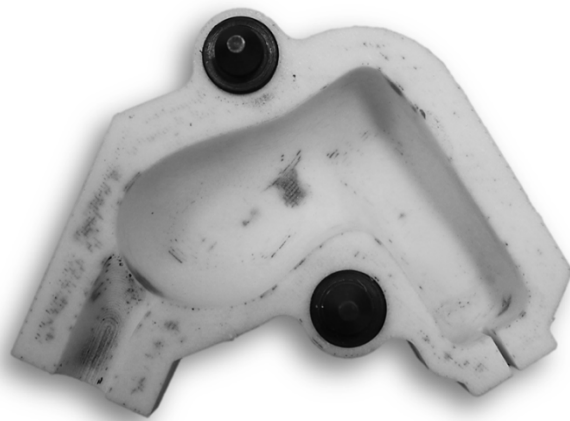
Figure 9. Mold cavity after injection of 20 parts.
