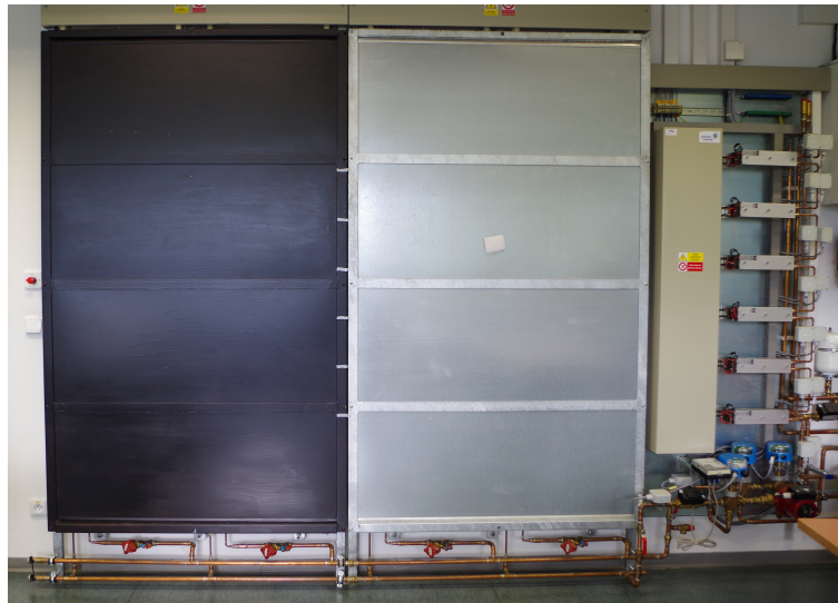
Figure 3. Accumulation device and thermoelectric assembly on the right.
