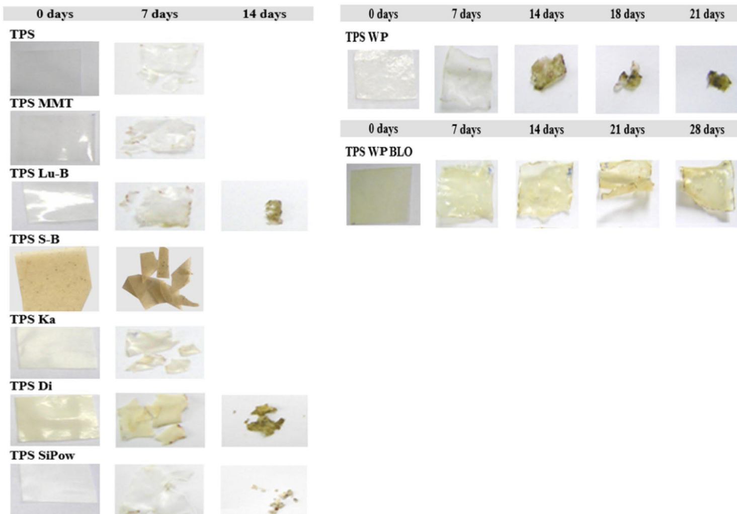
Fig. 4 Photographs of TPS and TPS/fillers before and after the biodegradation test (soil-burial test): TPS/clay blends - left; TPS/organic filler blends and hydrophobized TPS/organic filler blends - right. (TPS thermoplastic starch, TPS MMT thermoplastic starch/mont-morillonite Cloisite® Na + , TPS S-B thermoplastic starch/Sabenil® bentonite, TPS Lu-B thermoplastic starch/Lutila® bentonite, TPS Ka thermoplastic starch/kaolin, TPS SiPow thermoplastic starch/silica, TPS Di thermoplastic starch/diatomite, TPS WP thermoplastic starch/ waste paper, TPS WP BLO hydrophobized thermoplastic starch/waste paper)
