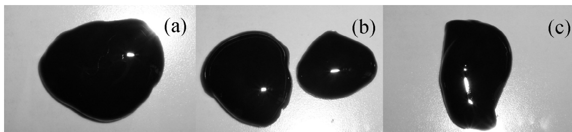
Scheme 2 The \text{Fe}^{3+} metal cross-linked gels at pH 12 (a) the cut gel (b) and recovered (c).
