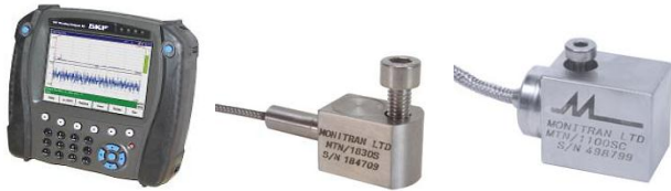
Figure 6. Measuring equipment (from the left side: FFT analyzer CMXA 80, accelerometers MTN/1830 and MTN/1100)
