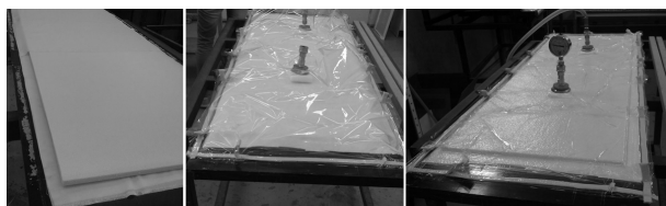
Fig. 10 Manufacturing process of sandwich structure using prepreg curing in the oven
