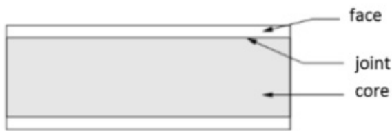
Fig. 4 The configuration of a typical sandwich structure
