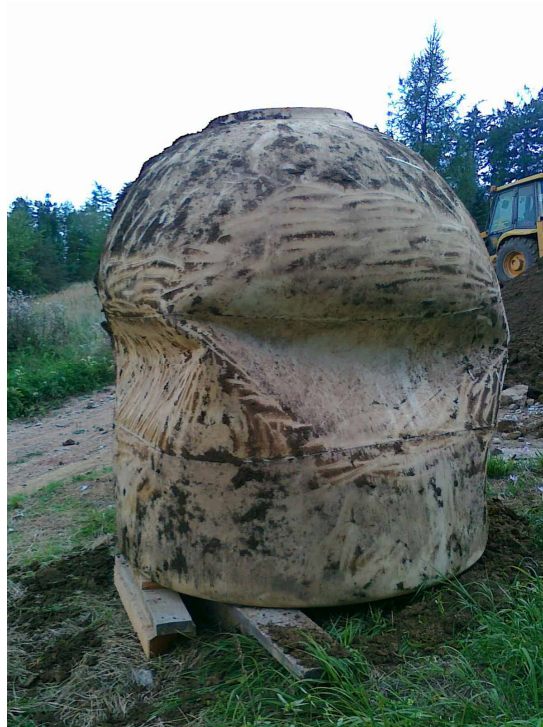
Figure 4. Example of loss of stability of an underground reservoir produced by rotomolding technology.
