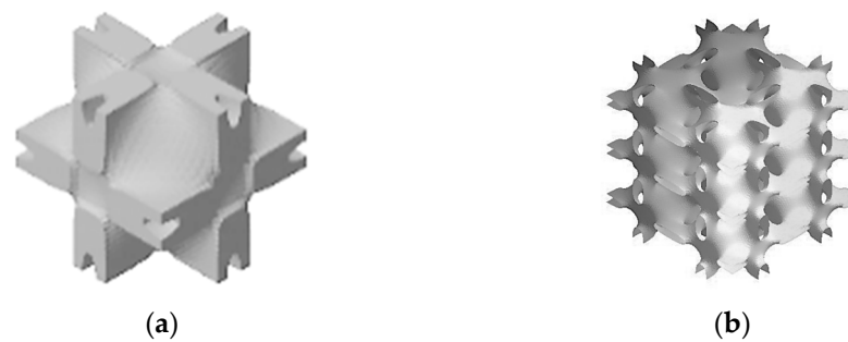
Figure 1. (a) The basic cell of the Neovius structure and (b) the complete Neovius surface.
