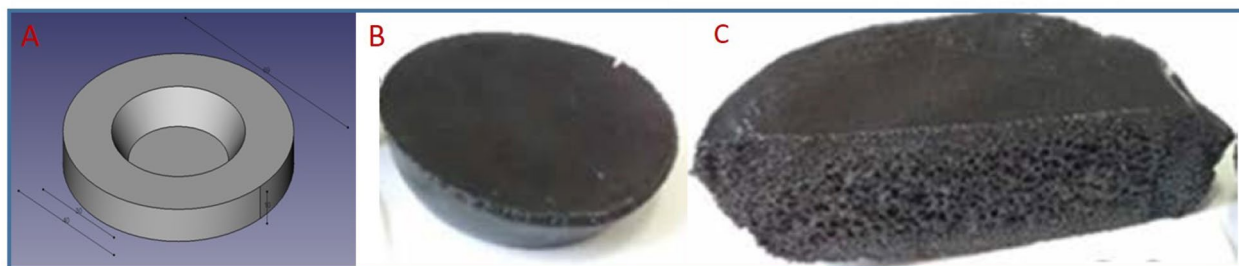
Fig. 1 The shaping form (A), the sample before foaming in an oven (B), and a prepared Foam 1 (C)
