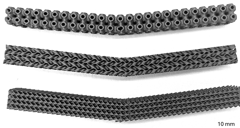
Figure 17. Cellular specimens after failure.
