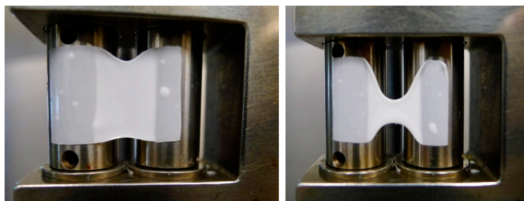
Figure 6. Deformation of REF rectangular samples: at 140 °C (left), and at 150 °C (right).
