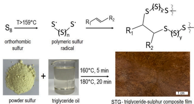
Fig. 1. Synthesis and processing of sulfur-triglyceride, and micrograph of resulting compression molded film.
