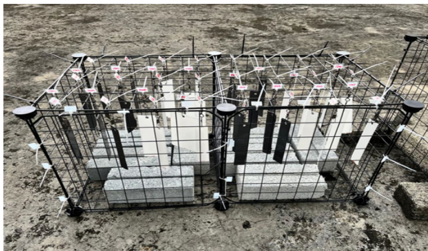
Fig. 2. Samples exposed to Kuala Lumpur's natural weathering.
